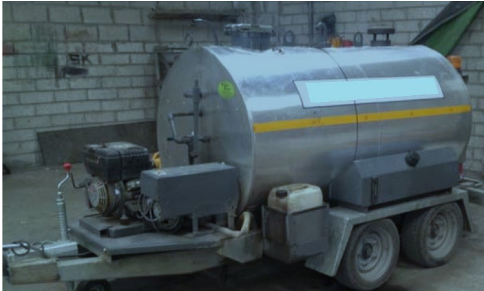
Figure 3-1: Towable Sprayer for Temporary Reinstatement
